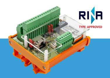
The NMEA Buffer is a specialized device that distributes NMEA or RS422 signals from a one transmitter to up to 12 listeners. It ensures galvanic isolation between the transmitted signal, power supply and listeners. Unit can operate with signal speed up to 230400 bps and power supply range from 9 to 36 VDC. The device has three functional modes: Dual Input Independent Transmission, Single Input Transmission, and Selectable Dual Input mode, which are further explained in this manual.
